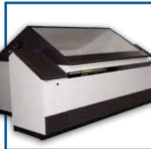
2 Salt Spray Corrosion
