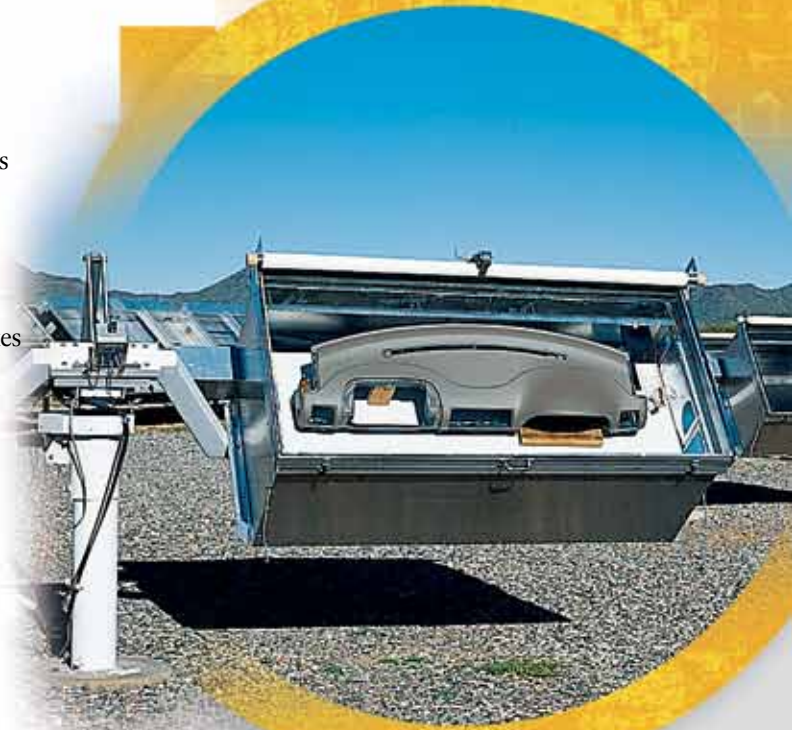
IP/DP Box Atlas Weather Station
